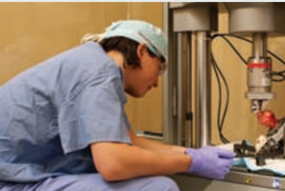
Olivier van der Meijden, M.D., working with the Instron ElectroPuls E10000, an electric-powered tensile testing machine.
